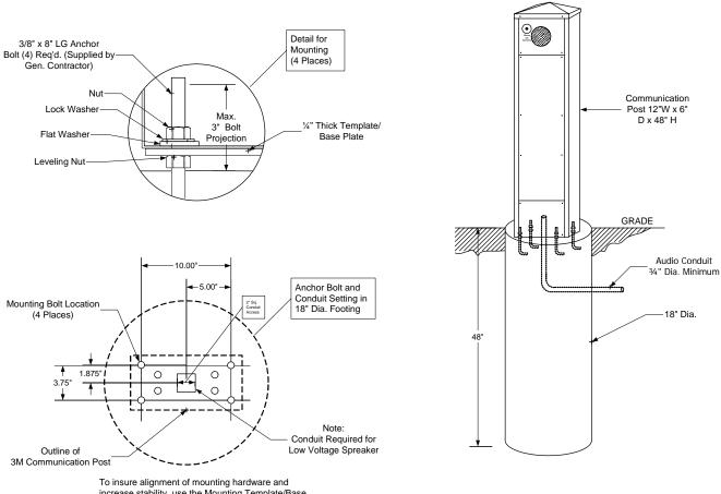
increase stability, use the Mounting Template/Base Plate provided as template and base platform
